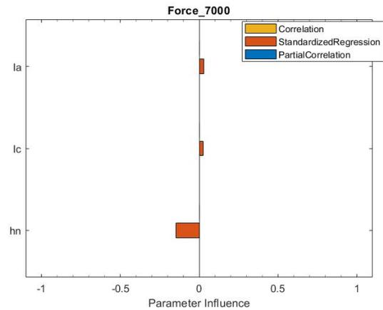
Figure 6 – Tornado plot indicating parameter influence (hn- NdFeB height, la- Length of AlNiCo, lc- Width of casing)
