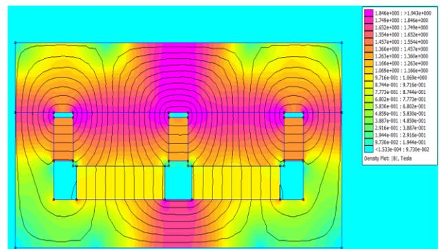
Figure 9 – EPMC in ON configuration
