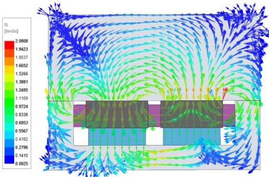
Figure 14 - Flux flow lines in ON configuration
