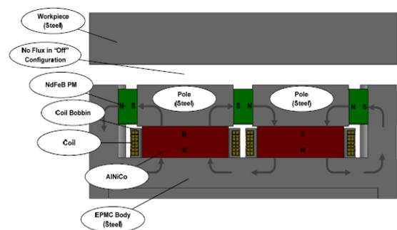
Figure 1 – EPMC device in OFF Configuration
