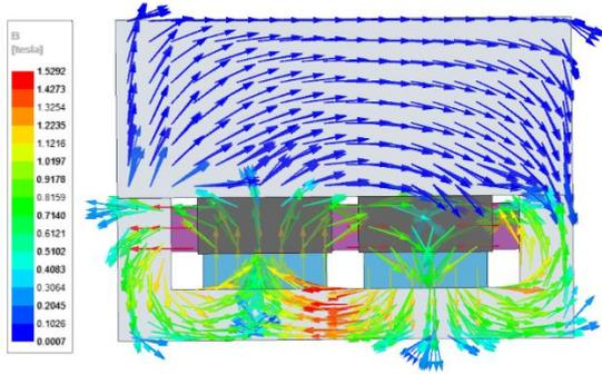
Figure 13- Flux flow lines in OFF configuration
