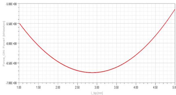
Figure 12 – Force in ON condition vs Ltop
