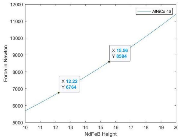
Figure 5 – Force vs NdFeB height results using MCA
