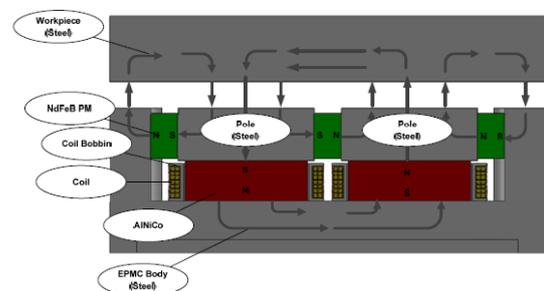
Figure 2- EPMC device in ON configuration
