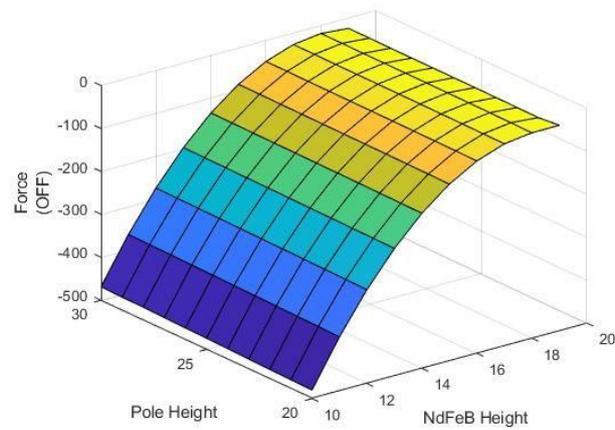
Figure 7 – Surface plot of Force (OFF) vs NdFeB height vs Pole height
