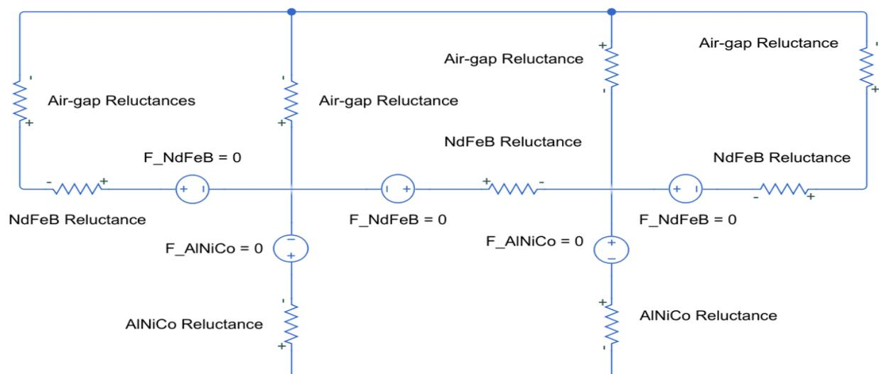
Figure 4- Magnetic Circuit for ON configuration
