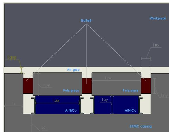
Figure 3- Cross-sectional layout of the clamp
